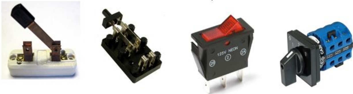
Plate 1: Knife Switch (SPST) Plate 2: Knife Switch (DPDT) Plate 3: Rocker Switch (SPDT) Plate 4: Rotary Switch (3P3T)
